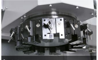
**T type turret** Servodriven with hydraulic locking system and ROMI disc for 12 fixed tools (ROMI VTL 500R / VTL 500L / VTL 700R / VTL 700L).
